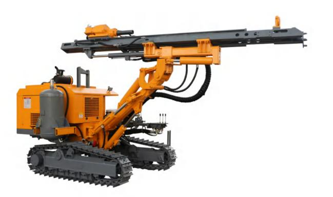
The integrated open-air DTH drill carriage is a drilling equipment that integrates the DTH drilling system and the screw air compression system.
